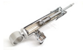
Adjustable damping force shock absorber with a proportional solenoid
