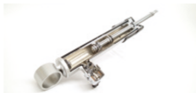
Variable damping shock absorbers with proportional solenoids
