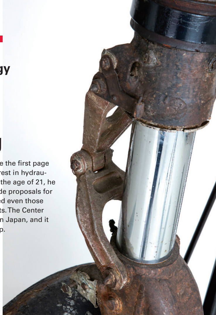
Invention of the Hydraulic Damper for Aircraft In 1935, Shiro Kayaba founded Kayaba Manufacturing Co., Ltd., where he invented the predecessor to the automotive shock absorber, the hydraulic damper (oleo strut) for aircraft. This invention set the course for KAYABA's current hydraulic technology, which can accurately control machinery that exerts several tons of force and absorb vibration to the optimum levels.
