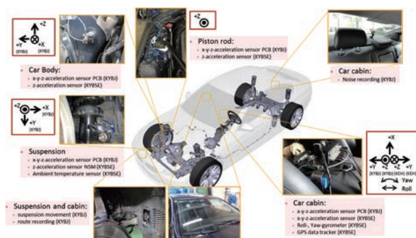
Fig. 3 Sensor positions inside the test vehicle for shock absorber oil evaluation tests at KYB Suspensions Europe S.A.
