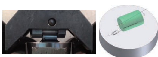
Fig. 2 Standard inclined roller in SRV ® tribometer
