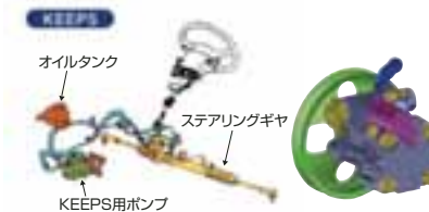
KEEPS: Kayaba Electronic Controlled Energy saving Power Steering
