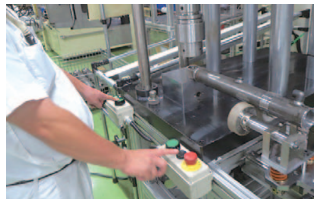
Install two-handed switches as a countermeasure to being caught in machinery
