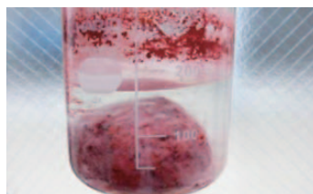
Waste paints and their water content are separated, and the water is treated appropriately and then discharged.
