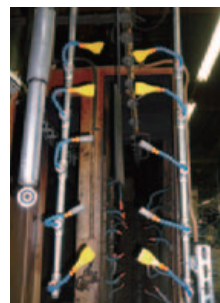
Coating equipment and compressed air blower nozzles
