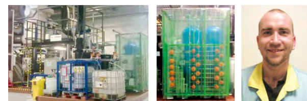
Ion exchange system Ion exchange resin unit Production Engineering Dept. Tomáš Jelínek
