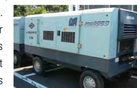
The engine compressor installed
