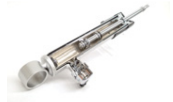
Adjustable damping force shock absorber with a proportional solenoid
