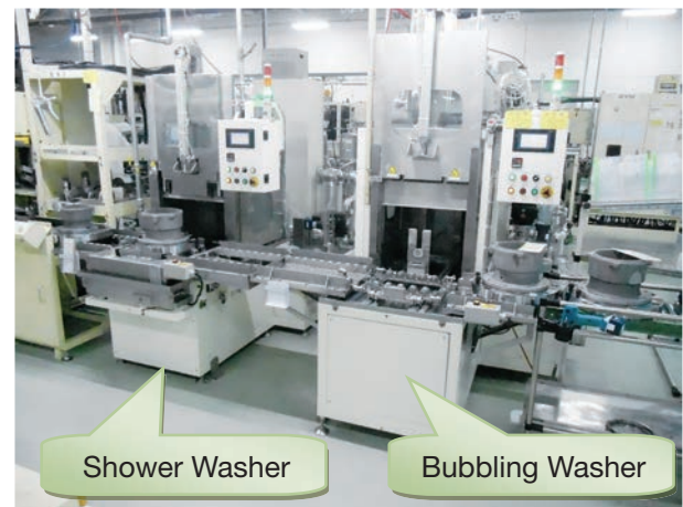
Photo 6 Bubbling Washer Appearance
