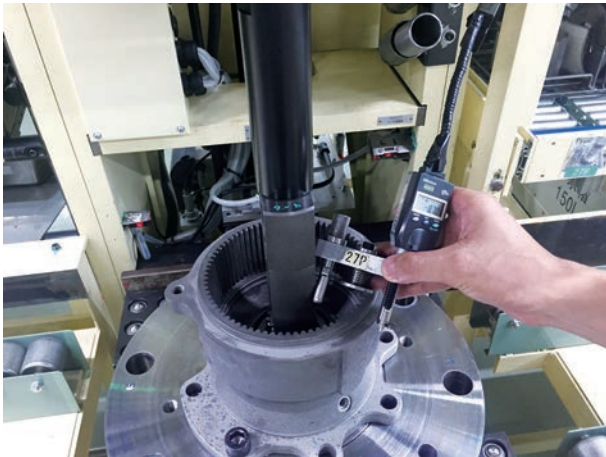
Photo 3 Clearance Measuring Apparatus
