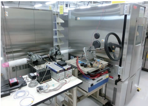
Photo 7 ECU operation confirmation test in low temperatures
