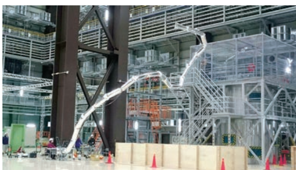
Fig. 2 20m-long robot arm (Taking on the “impossible” challenge)
