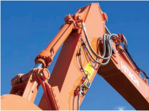
Fig. 6 Developed stroke sensing cylinder
