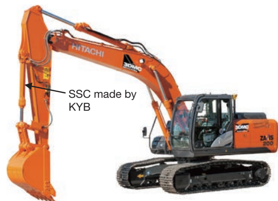
Fig. 2 ICT excavator ZX200X-5B made by Hitachi Construction Machinery
