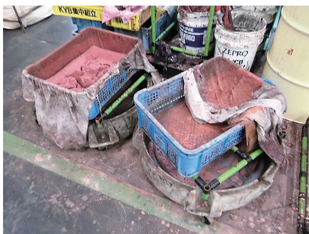
Photo 8 Filtering device I made from waste
