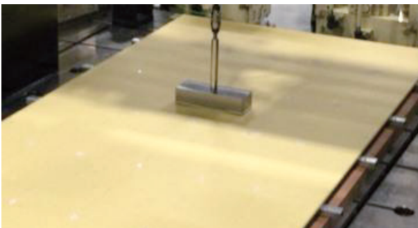
Photo 5 Measurement of static breaking load on ceiling
