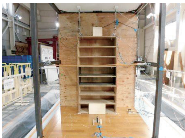
Photo 2 3-axis shaking table test
