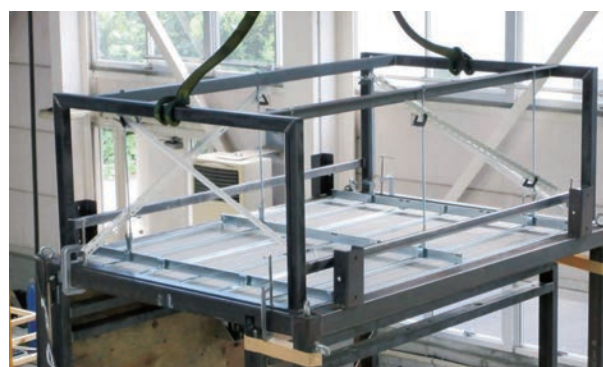
Photo 4 Simulated office building ceiling
