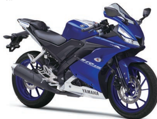
Photo 4 YZF-R15 Note 5) equipped with \varnothing 37 inverted FF (Source: Yamaha Motor Co., Ltd. Website)
