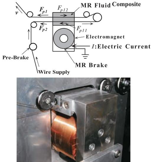
**Fig. 8** MR fluid porous composite brake developed for wire tension control system for coil winding
