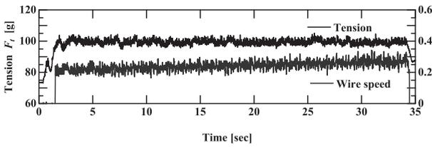
(b) Wire tension controller using MR fluid porous composite brake applied with PID tension feedback control
