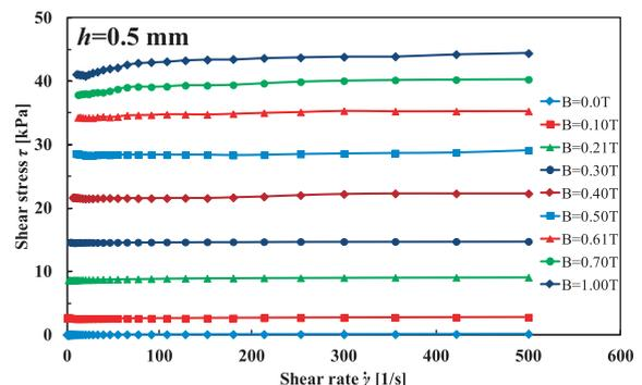
Fig. 2 Flow curves of MR fluid (MRF-132DG)
