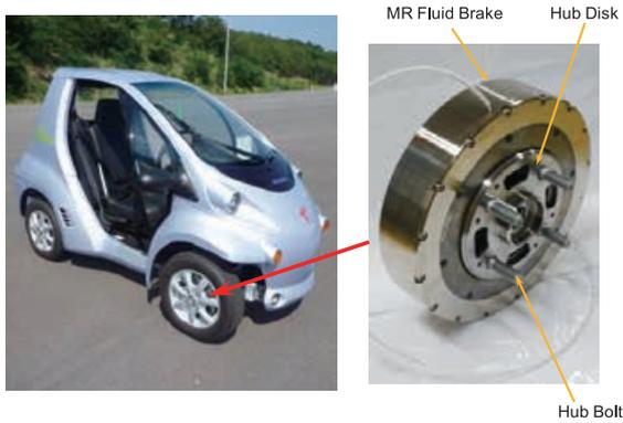
**Fig. 6** MR fluid brake for vehicles and its installation on a compact EV
