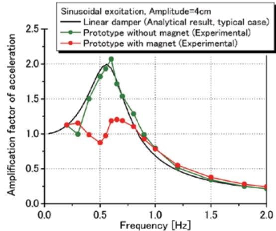
**Fig. 4** Seismic control property of SDOF base isolation system consisting of the developed MR dampers
