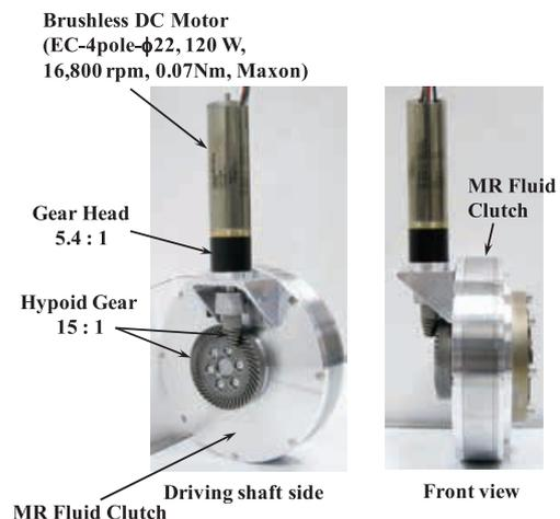
**Fig. 5** MR fluid actuator developed for use in power-assisted leg orthosis
