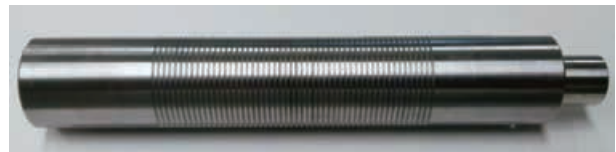
Photo 1 Appearance of piston rod prototype before plating
