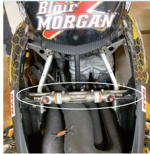
Fig. 9 Remote Reservoirs of Front Shocks were fixed in the hood
