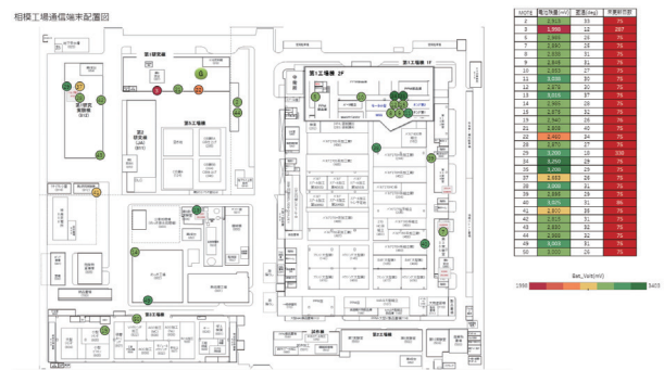
Fig. 10 Layout of sensor communication terminals and their battery status
