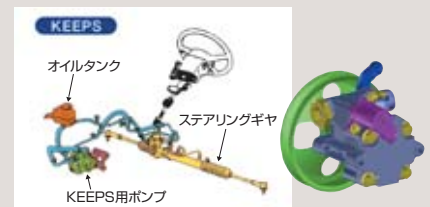
KEEPS : Kayaba Electronic Controlled Energy saving Power Steering
