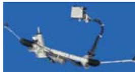
The assist power of the motor is controlled according to the steering power of the driver to realize optimal steering with the needed amount of assistance at the needed time.
