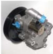
This pump is expected to be adopted in energy-saving steering systems such as large-size vehicles, SUV's and trucks that are difficult in applying EPS.
