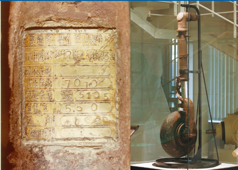
The metal plating of oleo struts on the sliding components of a Japanese Zero fighter plane discovered on the bottom of Japan’s Seto Inland Sea in 1977 was still shiny after more than 30 years underwater, demonstrating the sophistication of KYB’s technologies.
