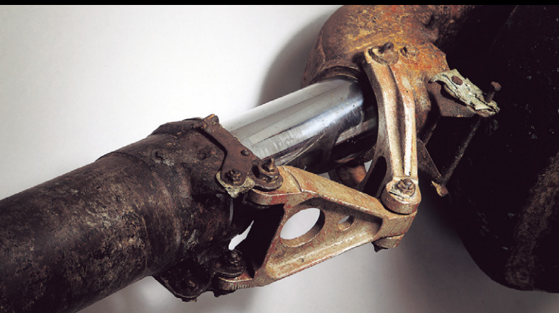
The metal plating of oleo struts on the sliding components of a Japanese Zero fighter plane discovered on the bottom of Japan’s Seto Inland Sea in 1977 was still shiny after more than 30 years underwater, demonstrating the sophistication of KYB’s technologies.
