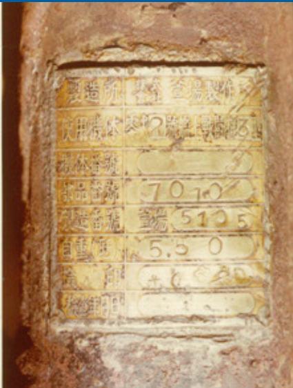
The metal plating of oleo struts on the sliding components of a Japanese Zero fighter plane discovered on the bottom of Japan’s Seto Inland Sea in 1977 was still shiny after more than 30 years underwater, demonstrating the sophistication of KYB’s technologies.
