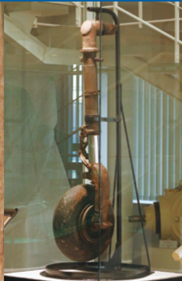
The metal plating of oleo struts on the sliding components of a Japanese Zero fighter plane discovered on the bottom of Japan’s Seto Inland Sea in 1977 was still shiny after more than 30 years underwater, demonstrating the sophistication of KYB’s technologies.
