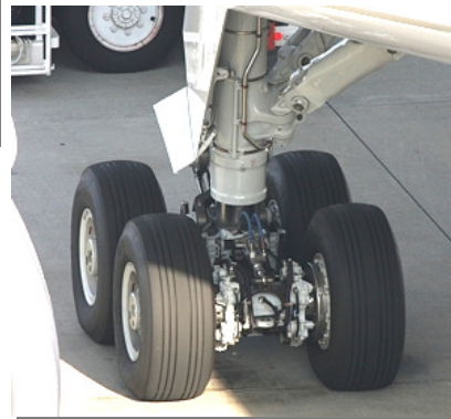
Actuator for opening and closing wheel well (nose landing gear)
