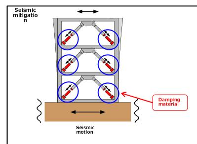
**Structure of** <u>mitigating vibration of the</u> <u>building</u> by wind or earthquake by placing damping materials on each floor
