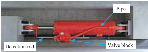
Photo 2 Appearance of a seismic isolation damper for narrow land
