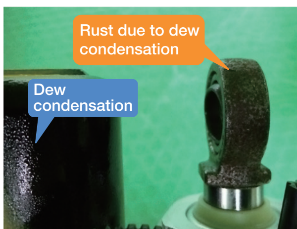
Photo 11 Dew condensation and rust of workpiece
