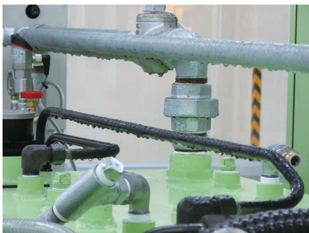
Photo 12 Dew condensation of hydraulic pipe
