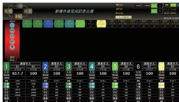
Fig. 3 Operation screen for K-compo SystemM
