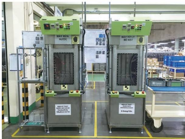
Photo 13 Preprocessing cleaner (Right: Preprocessing, Left: Cleaning)
