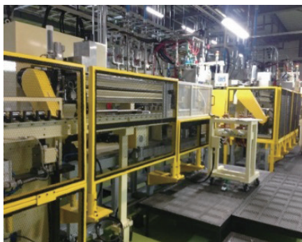
Photo 8 High-frequency hardening and tempering
