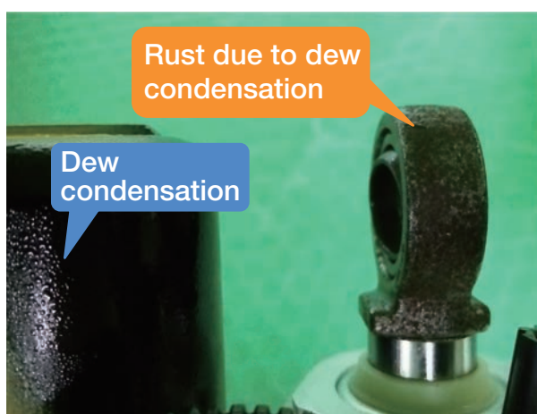
Photo 11 Dew condensation and rust of workpiece
