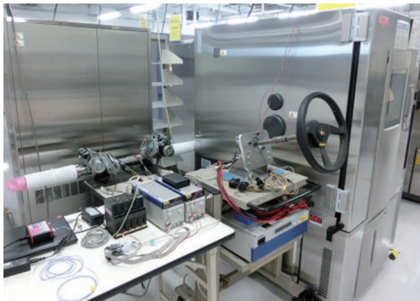
Photo 7 ECU operation confirmation test in low temperatures
