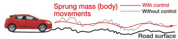
**Fig. 5** Road surface follow-up control image diagram
