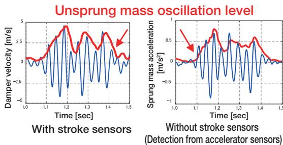
Fig. 7 Unsprung mass oscillation detection
