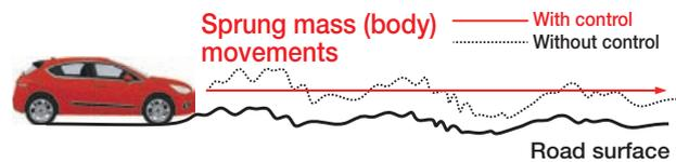
**Fig. 4** Comfort control image diagram
