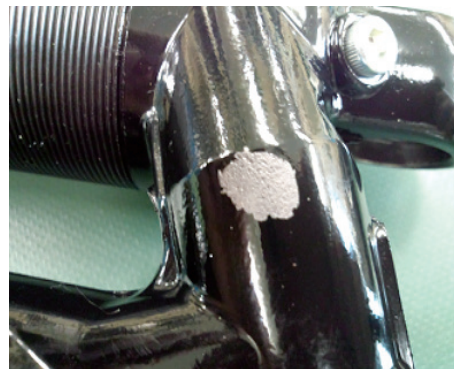
Photo 1 Exfoliation (aluminum material)
