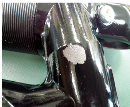
Photo 1 Exfoliation (aluminum material)
