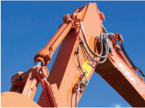
Fig. 6 Developed stroke sensing cylinder
