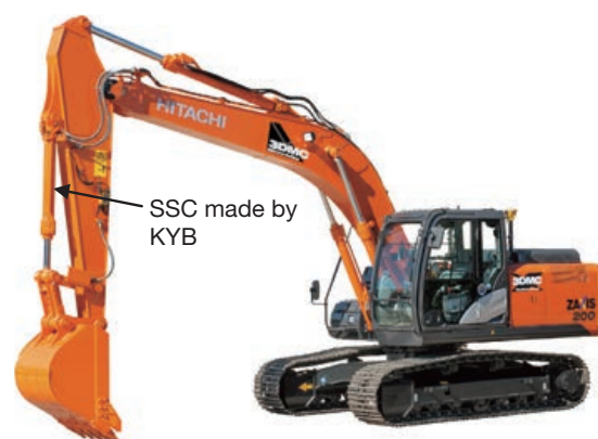
Fig. 2 ICT excavator ZX200X-5B made by Hitachi Construction Machinery
