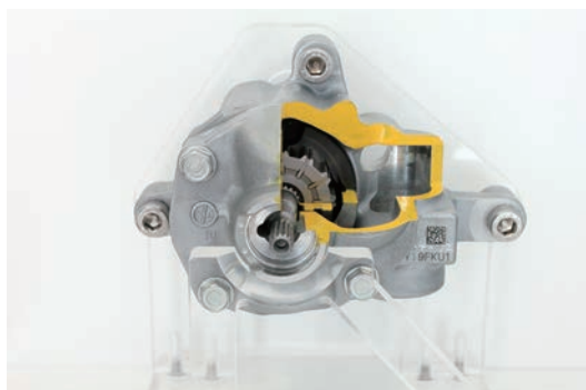
Photo 1 CVT vane pump (7K3)
