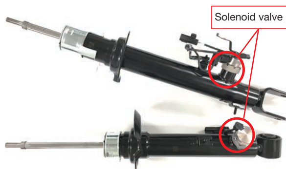
Fig. 4 Appearance of damping force adjustable SA with external SOL
