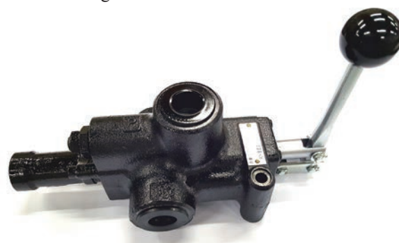
Photo 2 Appearance of control valve
