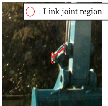
Fig. 3 Link joint region
