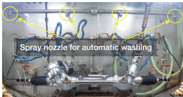
Photo 2 Internal of muddy salt water endurance test machine
