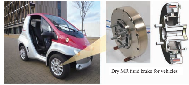
Fig. 14 Compact EV with dry MR fluid brakes on the four wheels
