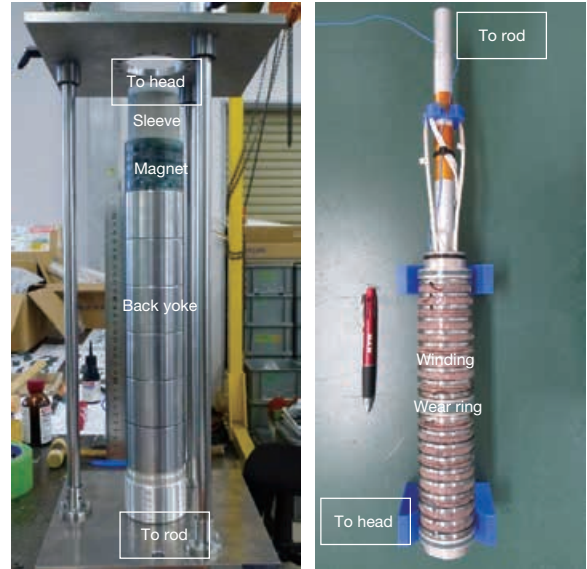
(a) Stator/magnet (being assembled) (b) Armature
