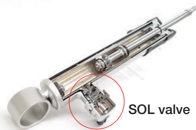
Photo 1 KYB adjustable SA with externally-mounted solenoid
