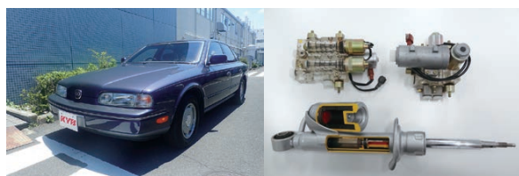
Photo 1 INFINITI Q45 (left) KYB hydraulic active suspension (right)
