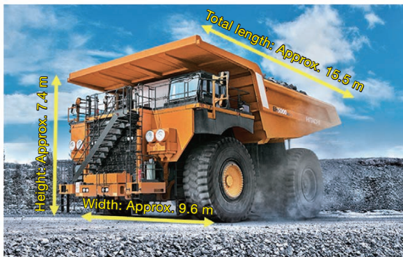
Photo 2 Appearance of EH5000AC-3 from Hitachi Construction Machinery (Reprinted from Hitachi Construction Machinery's website)
