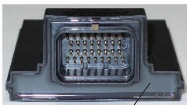
Photo 2 Filled with potting material
