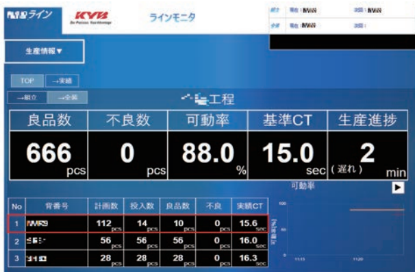
Fig. 3 Example of display on the line monitor screen (sample data shown)
