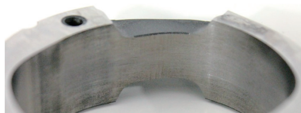
Photo 2 Cam ring with PV value lower than the limit after durability test
