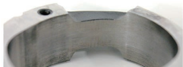
Photo 2 Cam ring with PV value lower than the limit after durability test
