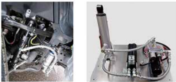
Photo 7 Damping adjustable SA for front wheels, height adjustable SA for rear wheels
