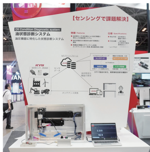
Photo 3 Oil condition diagnosis system (sensing, <experience-based sales> service)
