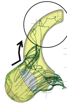
Fig. 12 Flow lines of suction oil passage before improvement
