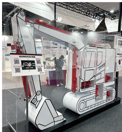
Photo 2 Mini excavator mock-up model (including hydraulic equipment for construction machinery)
