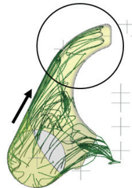
Fig. 16 Flow lines of suction oil passage after improvement
