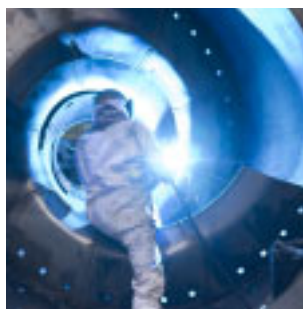
Welding operation on rotating drum for concrete mixer truck
