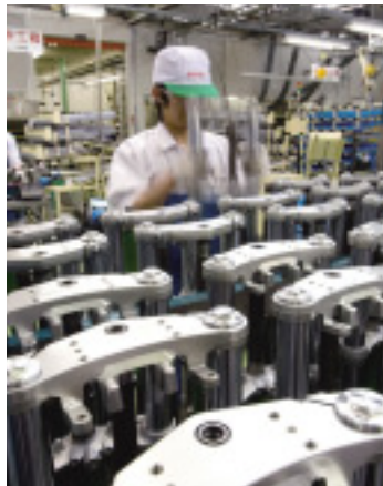
Bench test of front forks
