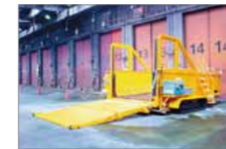
自走式コンベアごみ投入検査機 Self-Propelled Type, Foreign Material in Refuse Inspection Machine with Conveyor
